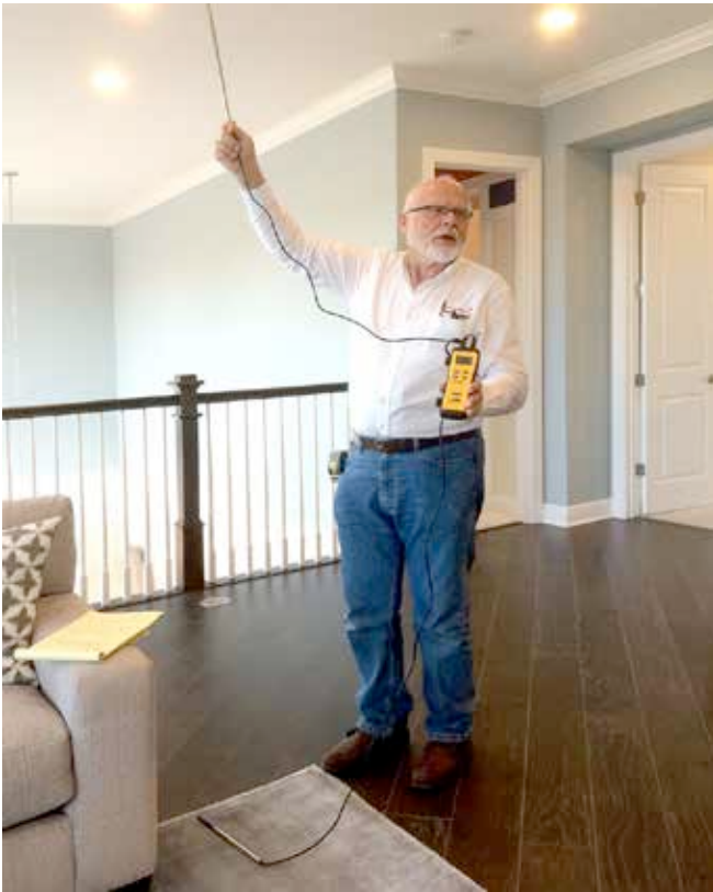
Photograph 10: Friend With Meter —Boys and girls you can do this experiment at home. First, find a friend who likes you but believes that you are wrong and brings his own dewpoint meter to demonstrate that you are clearly wrong. Sensor at floor and near ceiling.
